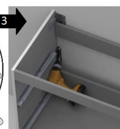
3 Fix the additional support to the wall (screw and wall plug not provided)
