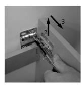
Push inwards with a screwdriver on the tongue, shaped flap, as shown in picture whilst lifting and pulling unit towards you.
