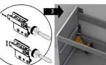
Fix the additional support to the wall (screw and wall plug not provided)
