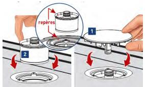
Place the water guard tube (2), position it by aligning the 2 marks (white raised triangle to orange triangle). Insert the cover (1).
