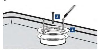
Tighten the stainless steel plate (4) on the drain body (6) with the 3 screws (3)
