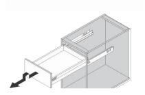
Pull; when it is fully open lift and continue to pull gently, following the movement of the arrow.
